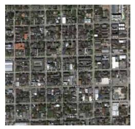
High Connectivity - Grid Link-Node Ratio - 2.2
