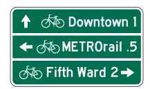
Figure 4.18 MUTCD Destination, Distance and Direction Signs.
