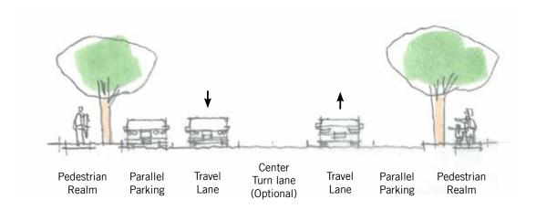
**Canal Street (65' ROW):** two or three-lane roadway with parallel on-street parking to support increases commercial development expected on the corridor.
