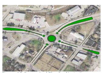
Figure 4.3 Conceptual Plan for Navigation Boulevard at York Street Roundabout
