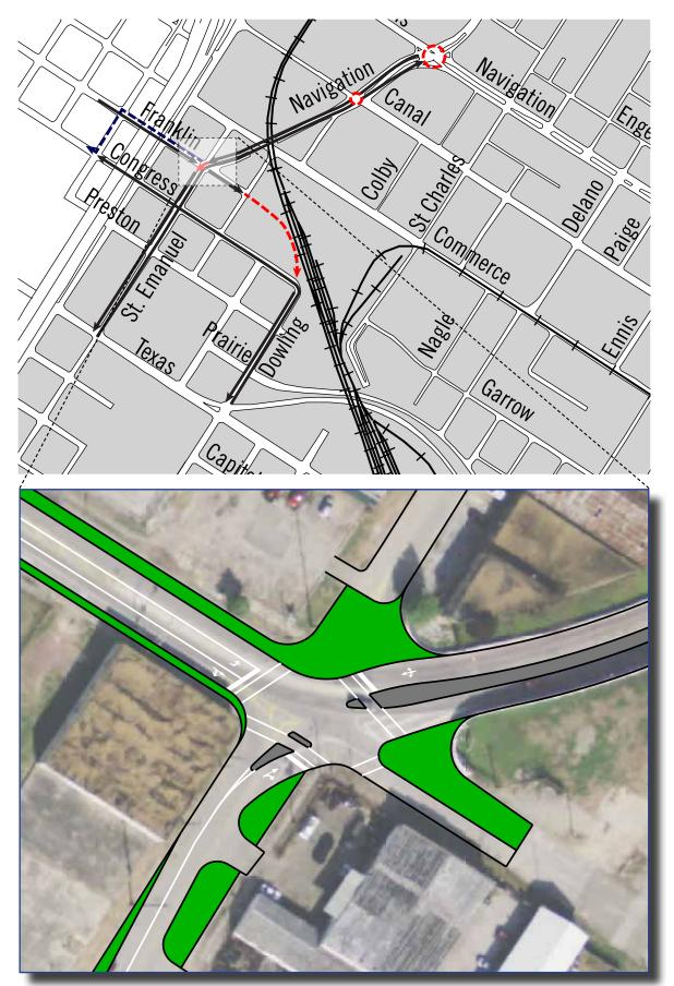
Figure 4.5 Potential Navigation Boulevard at St. Emanuel Intersection Realignment
