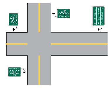
Figure 4.19 Typical sign placement at an intersection.
