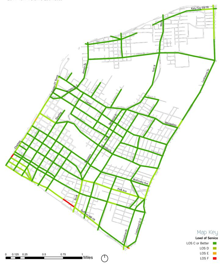
Figure 3.10 Travel Demand Model Volume-to-Capacity Ratio 2011 TDM Volume Estimates
