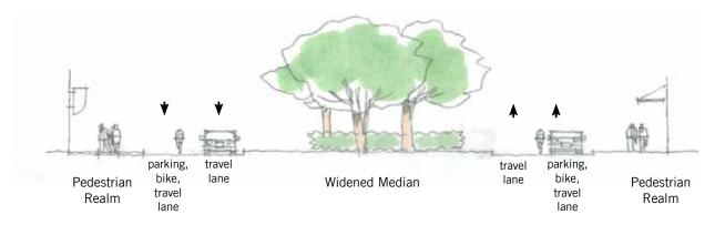
**Navigation Boulevard (120' ROW)**: four-lane boulevard section with median design to allow for both greater activation (St. Charles Street to Delano Street) and angled parking (Delano Street to Palmer Street).
