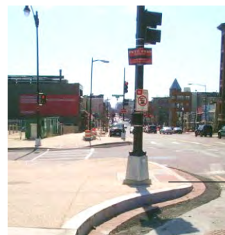
Pedestrian safety can be improved with the introduction of bulb-outs, which can help shorten pedestrian crossing distance, while also making them more visible.
