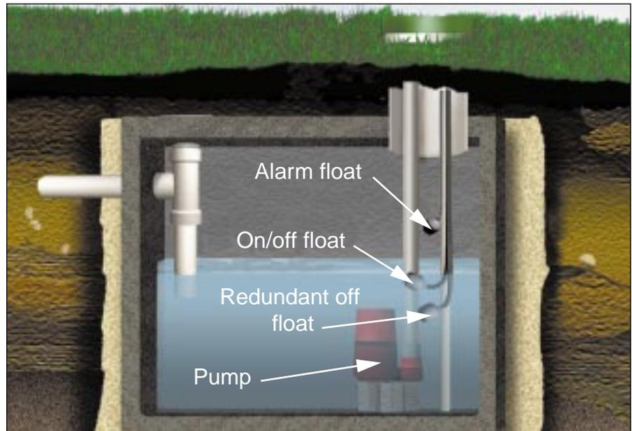
**Figure 2:** Floats in the pump tank signal the pump to start or stop dosing wastewater to the drain field.
