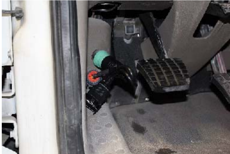
Figure 3. HEM Data Logger Installed on Vehicle.
