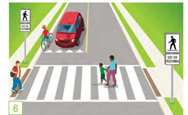
FIGURE 4.6 MIDBLOCK CROSSING SIGNAGE/ PAVEMENT MARKINGS, HOUSTON PARKS BOARD
