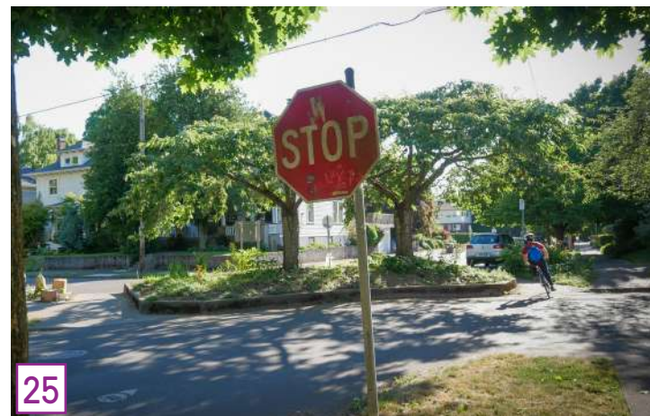
25 FIGURE 4.25 DIAGONAL DIVERTER, PORTLAND, OR
