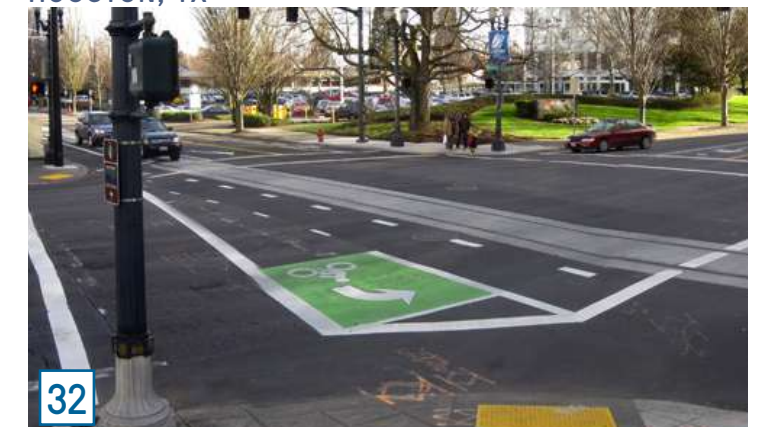
FIGURE 4.32 TWO-STAGE TURN BOX, PORTLAND, OR
