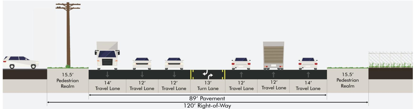
**Figure 3.3** Typical 7 Lane Cross-section - Northbound FM 1092 at Greenbriar Drive/Mula Road
