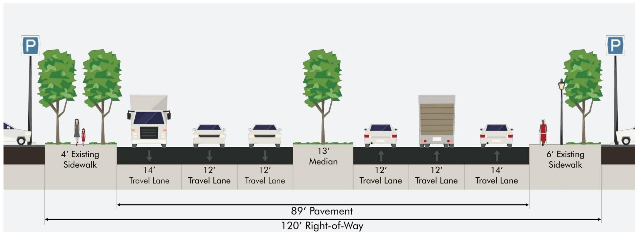
Figure 5.3 Proposed Alternative Cross-section - US 59 to Roark Road
