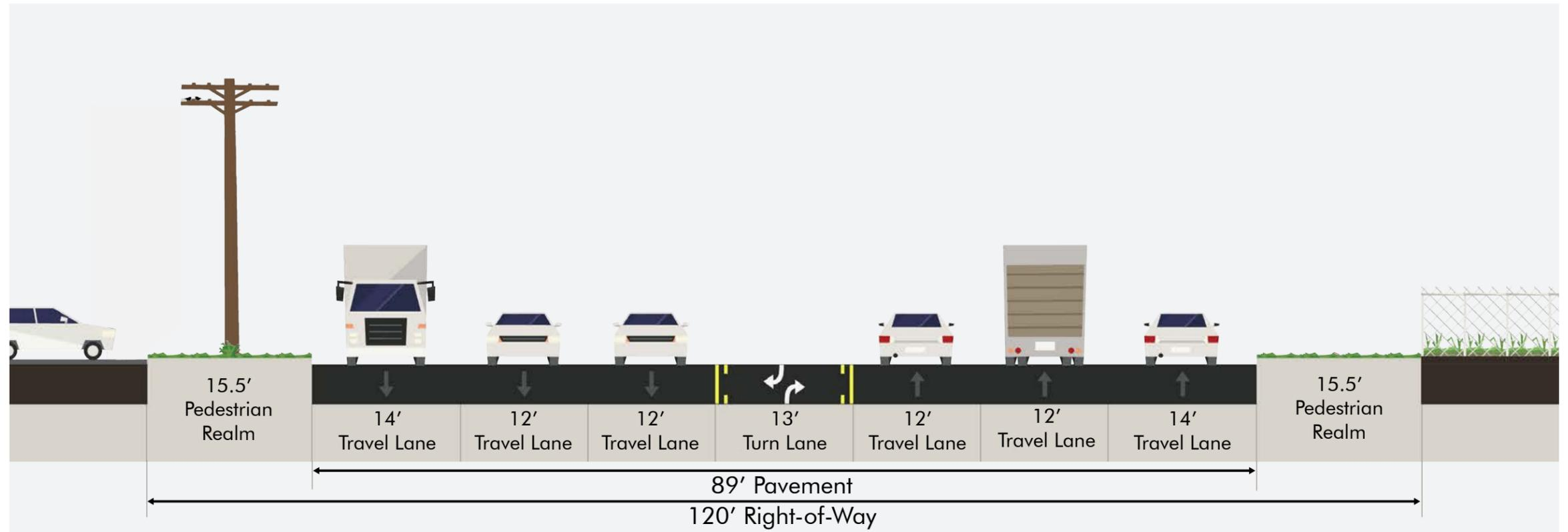
Figure ES.2 FM 1092 Study Corridor Typical Cross Section
