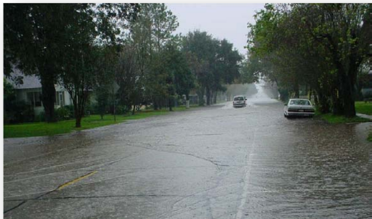
Figure 33. A storm event has surpassed the design frequency for which the street was designed
