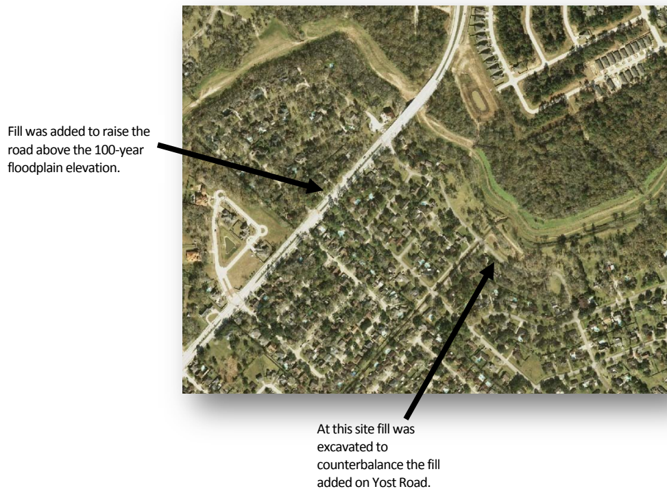
Figure 15. Overview of Pearland's Yost Road project
