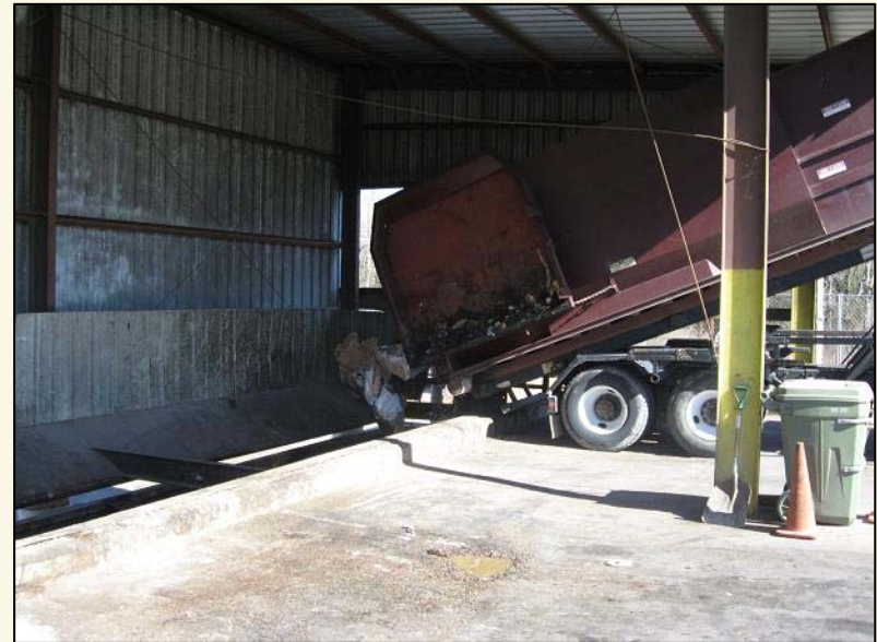
Direct Dump Into Open-Top Container
