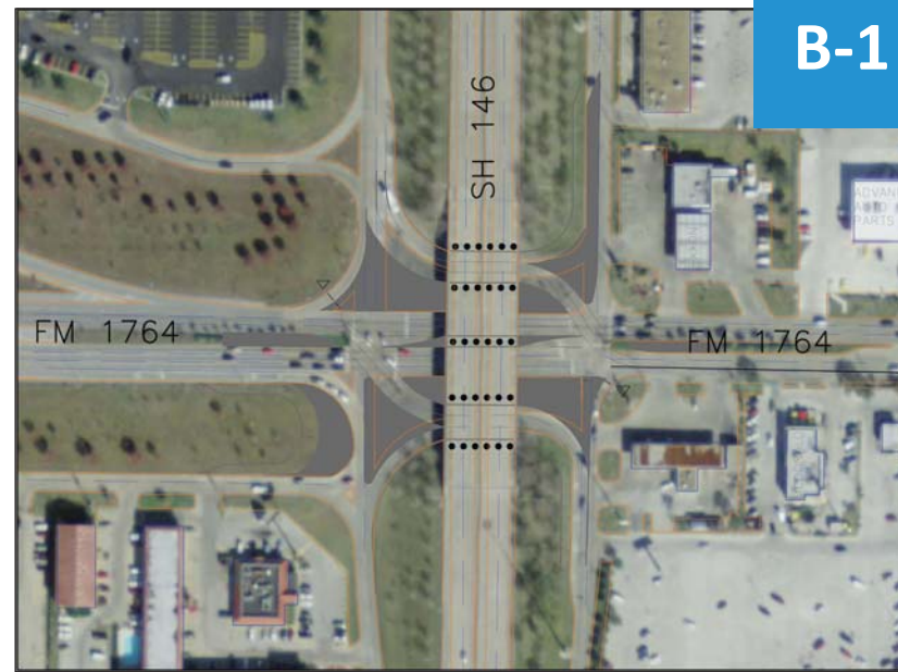
Figure C.2: SPUI configurations considered
