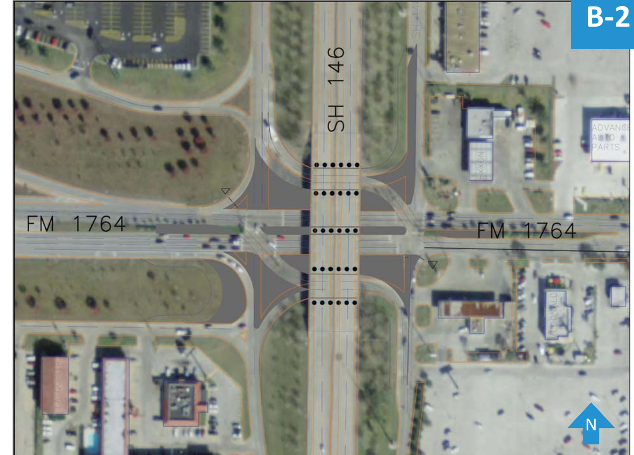
B-2: Similar to Alternative B-1 for the northbound and southbound left turns. However, the eastbound and westbound left turns would be routed from their current movement through the interchange. Westbound FM 1764 traffic heading south on SH 146 would pass straight through the interchange and take the ramp leading to the turnaround roadway under FM 1764 and then u-turn back to tie to the southbound service road south of FM 1764, turning right to proceed south. Eastbound FM 1764 traffic heading north on SH 146 would turn right in advance of the interchange to the southbound service road and another immediate right to the turnaround roadway under FM 1764, and then back to tie to the southbound service road north of FM 1764, entering the u-turn to proceed north on the northbound service road. This alternative reduces the most delay at the interchange, but adds mileage for the eastbound and westbound left turns, and the eastbound left-turn movement through the u-turn is cumbersome.
