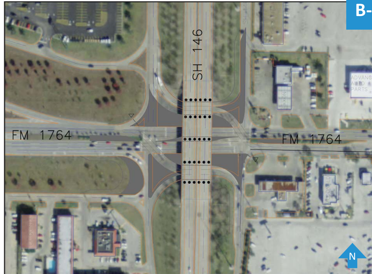
B-1: Similar to Alternative A-1, the northbound and southbound service roads' left turns would be realigned to allow them to move concurrently, reducing overlap delay. However, the realignment is shifted further to eliminate the use of the opposing lanes during the left turn movement. The eastbound and westbound left turns can be treated as in A-1 or as in A-2, with the A-2 configuration more effective at reducing delays.
