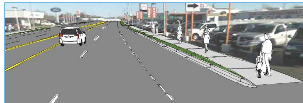
Figure 5.1: Continuous right-turn lane
