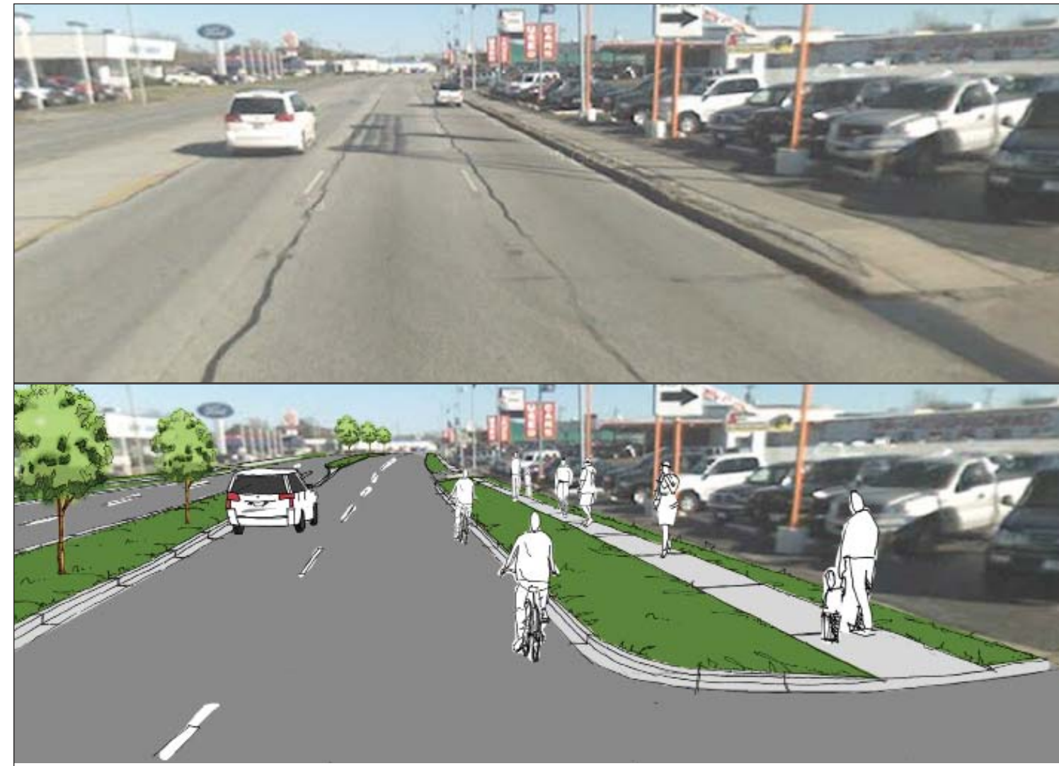
Figure 4.7: Roadway diet; before and after
