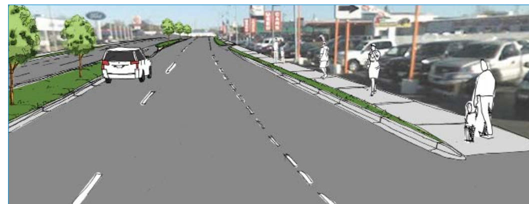
Figure 5.2: Raised median with optional landscaping
