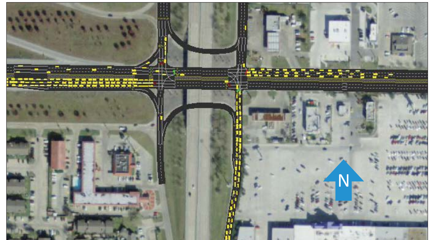
Figure 4.1: Extensive queue lengths and delays are experienced during the PM Peak Hour at the SH 146 interchange (screenshot from FNI's TransModeler simulation)
