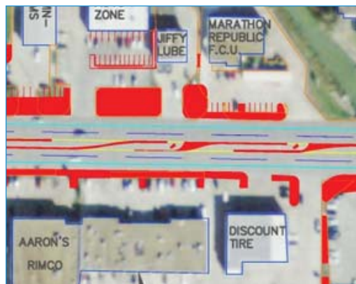
Sample access management tools, top to bottom, continuous right-turn lane, raised median with optional landscaping and driveway closures and merged parking areas.
