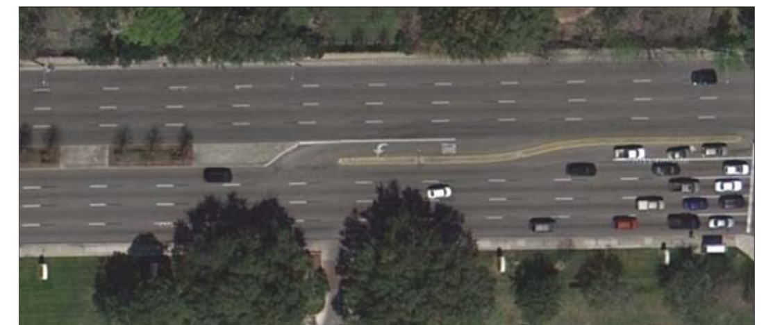
Figure 4.4: Channelized median left-turn lane (Westheimer Road, FM 1093, Houston)
