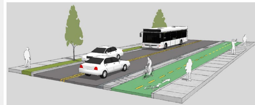
Figure 17.23 – BIDIRECTIONAL PROTECTED BIKE LANE WITH CAST-IN-PLACE CURB
