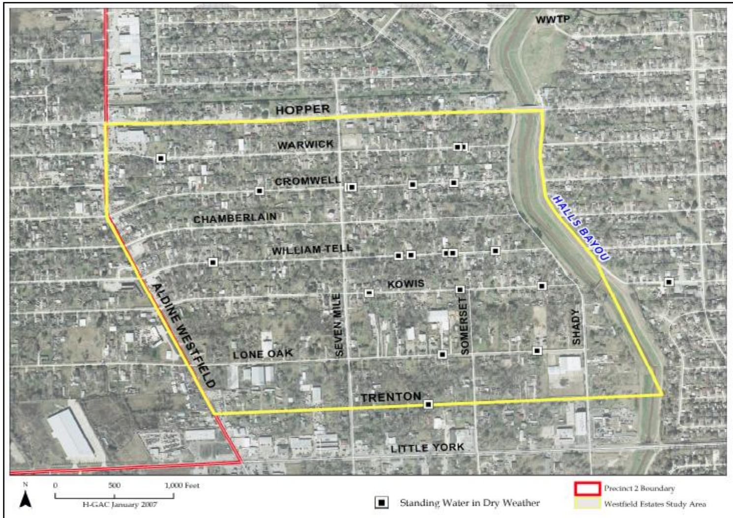
Figure 18: Dry Weather Standing Water Locations in Westfield Estates (Source: Data -HCPID; Mapping - Houston Galveston Area Council)
