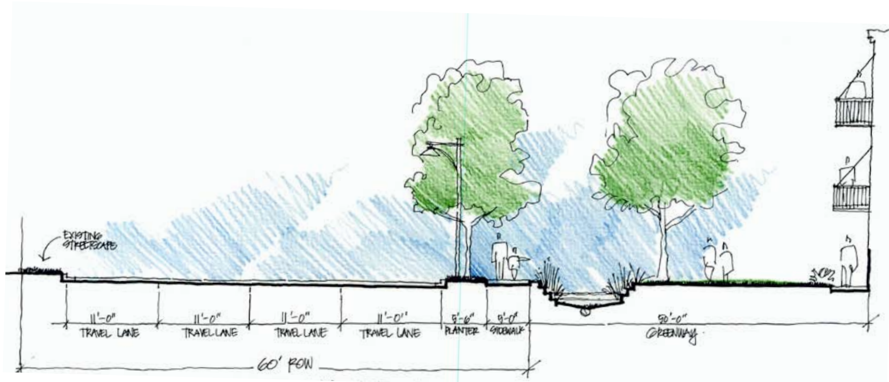
The Gillette Street ROW north of West Dallas widens to sixty feet and starts to serve more intense land uses, including the potential redevelopment of the Gillette Tract. This option shows a four-lane roadway (with the assumption that office, residential and commercial uses will be a part of the redevelopment), and a greenway that buffers new development, as well as connects pedestrians to Buffalo Bayou. The greenway and road should work together, providing maximum water quality and scenery.
