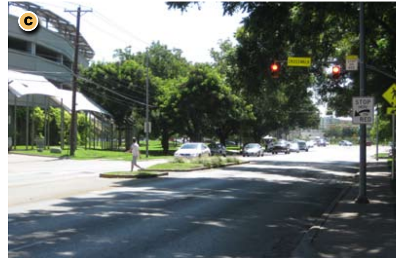
A fully-protected pedestrian crossing is ideal for high-traffic areas with regular pedestrian activity. Stop lights and signage increase visibility. Pedestrian crossings to the Bayou and downtown should be studied at the time of TxDot improvements to IH 45.
