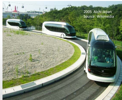
Toyota ITMS Automated Buses Following Magnetic Markers in Roadway at 2005 Aichi Expo
