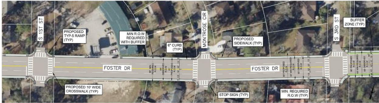
Figure 19 Foster Drive Proposed Schematic between S 1st St and S 3rd St
