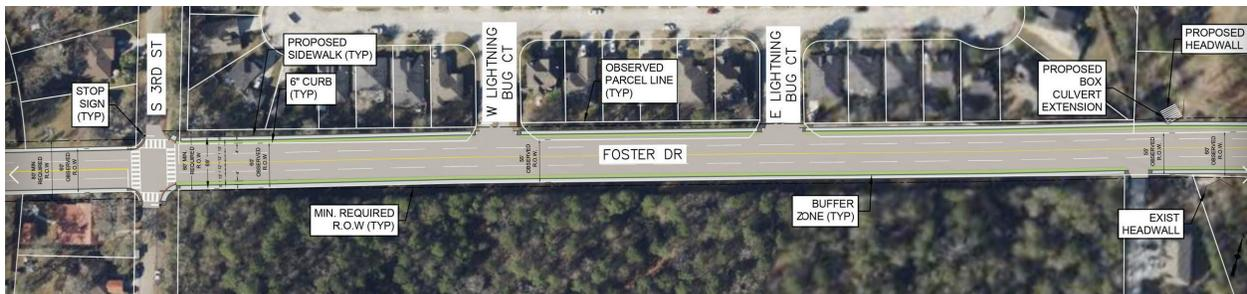
Figure 21 Foster Drive Proposed Schematic between S 3rd St to the Wetland
