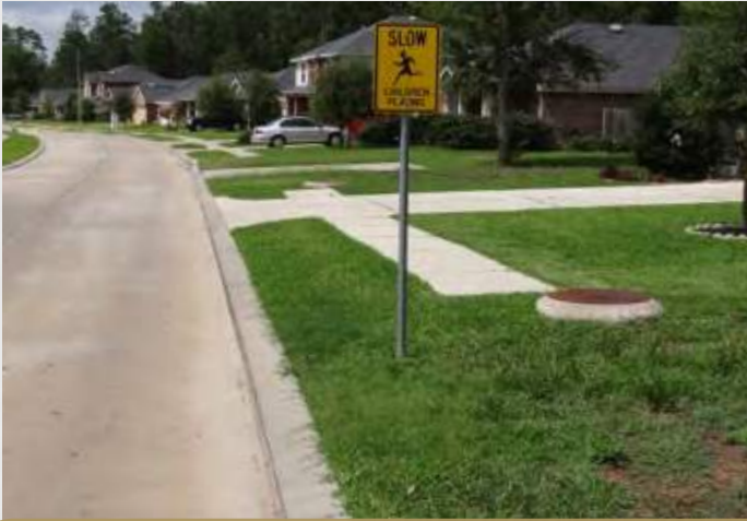
Sidewalks are ineffective if they do not create a continuous path to nearby destinations.
