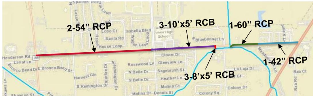
Figure 3. Proposed Storm Sewer System
