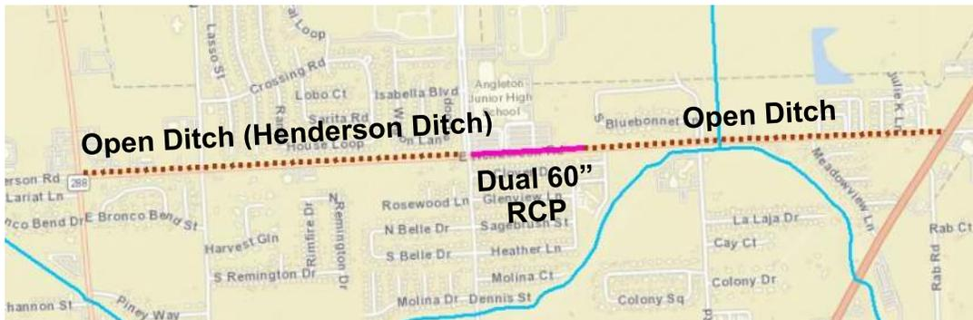
**Figure 2. Existing Drainage System**
